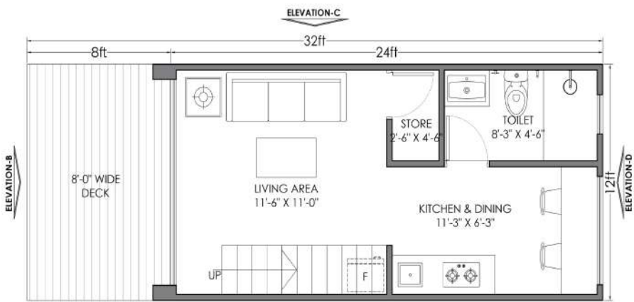
SMART HOUSE DOUBLE - A4 GROUND FLOOR PLAN COVERED AREA = 312 Sq. Ft DECK AREA = 72 Sq. Ft TOTAL BUILT AREA = 528 Sq. Ft
